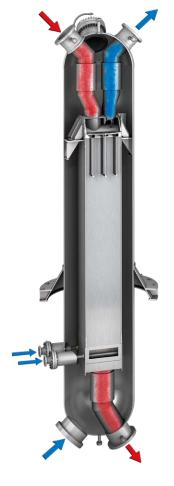
The liquid feed enters from the side, and thanks to the Spray Bars it is perfectly mixed with the recycle gas, which enters the heat exchanger at the bottom. The feed/gas mixture moves up through the plate pack while the reactor effluent travels in the opposite direction.
