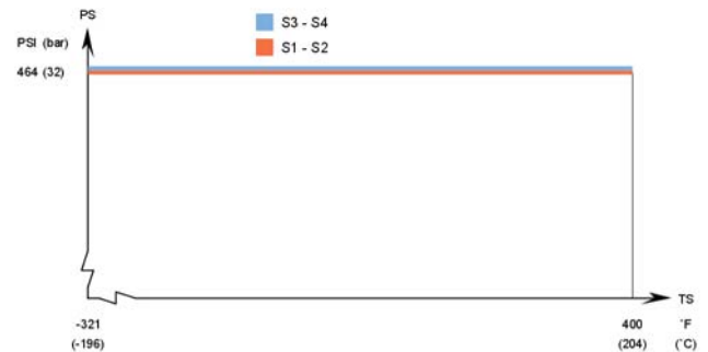
CB112AQ – UL approval pressure/temperature graph
